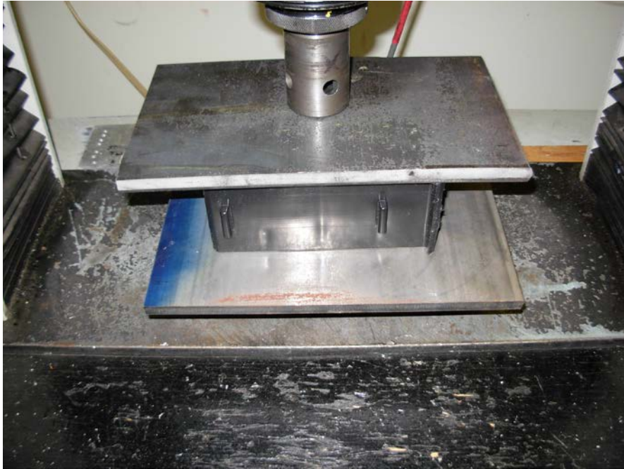
Figure 1 Load Test of Full Section
